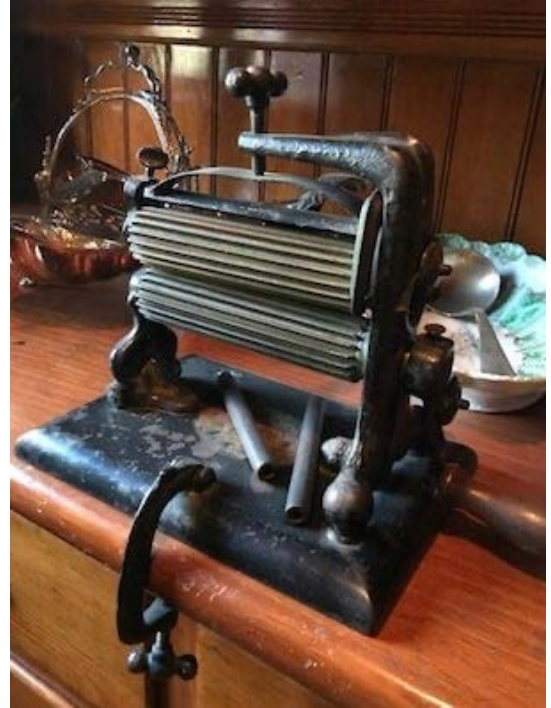
Rosson House pleating or crimping iron, used to press ruffles or pleats in clothing.
